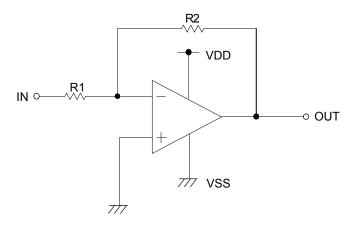
Figure 29. Inverting Amplifier Circuit
