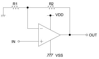
Figure 30. Non-inverting Amplifier Circuit
