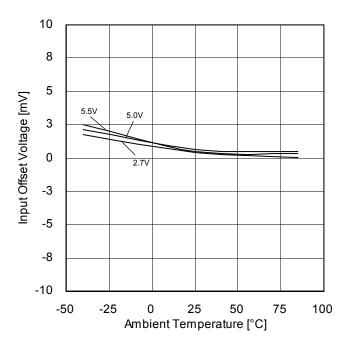
Figure 13. Input Offset Voltage vs Ambient Temperature ( $V_{ICM}$ = VDD,  $E_{\kappa}$ =-0.1V)
