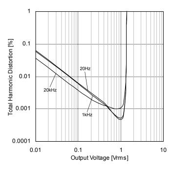
Figure 23. Total Harmonic Distortion—Output Voltage (VDD/VSS=+2.5V/-2.5V, Av=0dB,  $R_L$ =2k $\Omega$ , DIN-AUDIO,  $T_A$ =25 $^{\circ}$ C)
