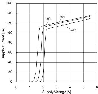
Figure 2. Supply Current vs Supply Voltage
