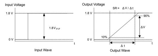
Figure 27. Slew Rate Input and Output Wave
