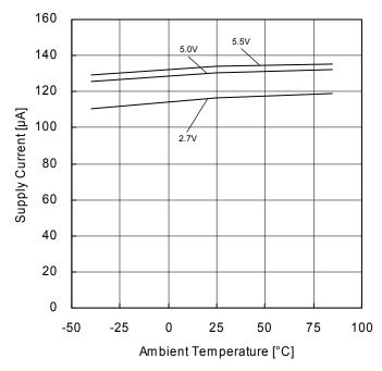
Figure 3. Supply Current vs Ambient Temperature
