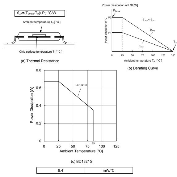
When using the unit above  $T_A$ =25°C, subtract the value above per degree °C. Permissible dissipation is the value when FR4 glass epoxy board 70mm × 1.6mm (copper foil area below 3%) is mounted
