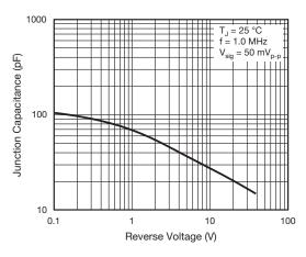
Fig. 5 - Typical Junction Capacitance
