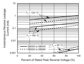
Fig. 4 - Typical Reverse Leakage Characteristics
