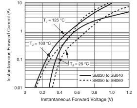
Fig. 3 - Typical Instantaneous Forward Characteristics
