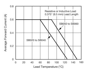
Fig. 1 - Forward Current Derating Curve
