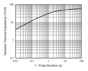
Fig. 6 - Transient Thermal Impedance
