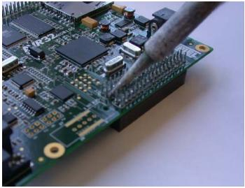
Figure 3-2. Soldering stack through headers to the NGW100
