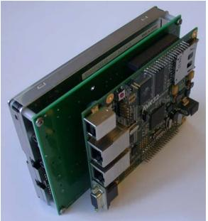
Figure 3-5. Assembled EVKLCD100 connected to a NGW100
