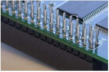
After all the pins on each header are properly soldered, the NGW100 is ready for use with the EVKLCD10X kit.
