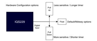
Figure 7.1 IQS229 configuration pin options
