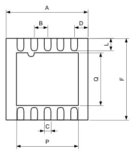
Figure 9.1 DFN-10 Package dimensions (bottom view)
