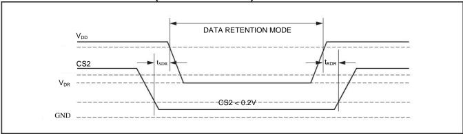
If CS1>VDD-0.2V, all other inputs including CS2 must meet this condition.
