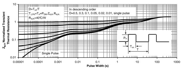
Figure 11: Normalized Maximum Transient Thermal Impedance
