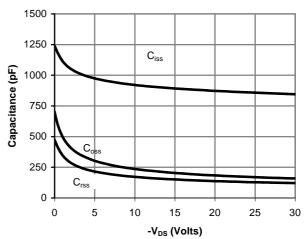
Figure 8: Capacitance Characteristics
