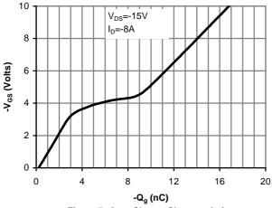
Figure 7: Gate-Charge Characteristics
