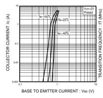
Fig.4 Grounded emitter propagation characteristics
