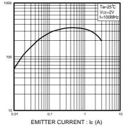
Fig.5 Gain bandwidth product vs. emitter current
