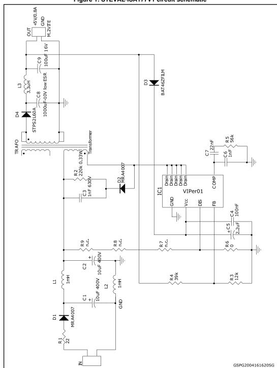
Figure 1: STEVAL-ISA177V1 circuit schematic
